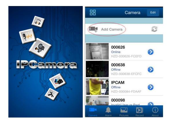
Click (Click here to add cameras) can search for a local area network cameras, select the search out of the camera can add this camera, enter the camera name, user name, password, and click OK, you can see the added cameras in the camera list; as follows Figure:
