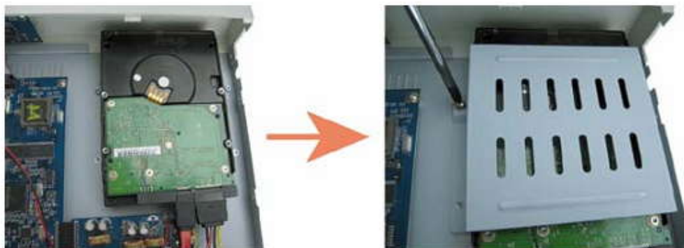
STEP4: Put the HDD and replace the bracket back
