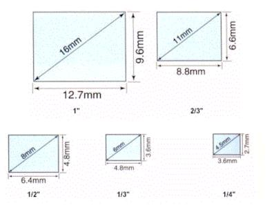
: A 1/2" format lens can be used with a camera having a 1/2" or a 1/3" imager; however it cannot be used with 2/3" or 1" format cameras.
