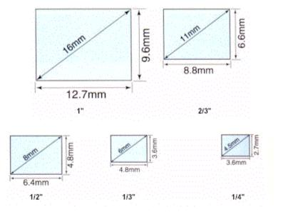
: A 1/2" format lens can be used with a camera having a 1/2" or a 1/3" imager; however it cannot be used with 2/3" or 1" format cameras.
